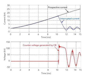
Figure 1 - Test results of active current injection HVDC circuit breaker at KEMA Laboratories
