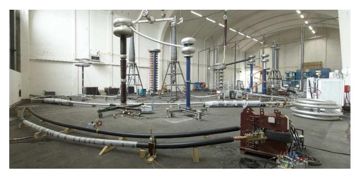
Two unique test requirements in testing a HVDC cable system compared to that of a HVAC cable system exist: a specified maximum temperature drop across the insulation of a cable and a superimposed impulse withstand test.
