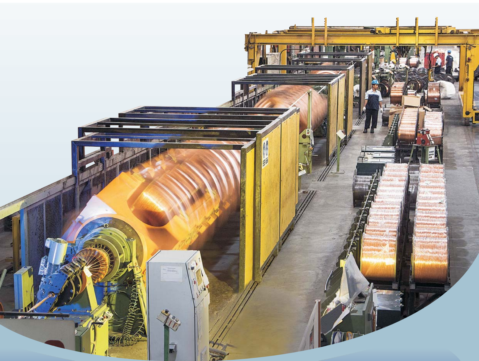
Conductor Stranding Process
